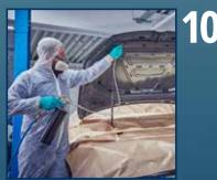
After treating the underbody, the cavities in the rear lid and bonnet must be sealed. Please ensure that the engine and boot are completely covered.
