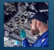
Next, the vehicle must be inspected. Flaking rust and all deposits must be removed. To do this, a rust remover such as **DINITROL Zero Rust Gel** can be used. The gel is applied to the rusted areas with a brush. Leave the gel on for 12-24 hours and then remove the loosened rust.
